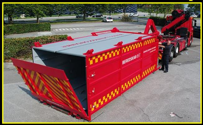
Container puts out inextinguishable fires in electric cars. (Link on Picture.)
